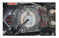
4. Remove the factory fog light assembly. Use a T20 Torx driver to remove the three screws. We recommend using hand tools to reduce the chance of thread stripping or heating of the plastic that may occur with power tools.
