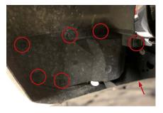
3. Remove the plastic fog light covers. To do so, use a 7mm socket and ratchet to remove the seven screws shown in the picture to the left.
