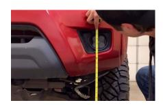
10. On your vehicle, measure the distance between the ground and the center of your SS3 pod. This is your mounting height.
